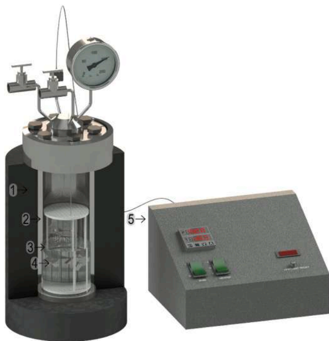
Fig. 2. Schematic arrangement for corrosion experiments in Parr pressure vessel. 1) Heating blanket; 2) Pressure vessel; 3) Specimen holder; 4) Specimens; 5) Temperature controller.
