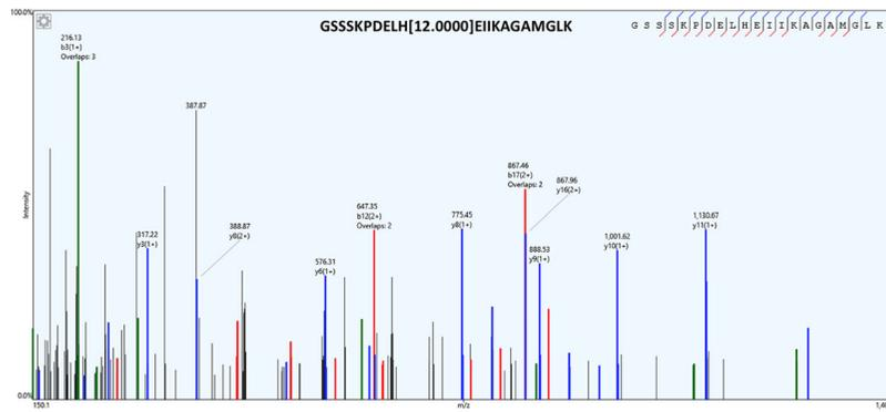
**Figure 4.** LC-MS/MS spectrum of the GSSSKPDELH[+12.0000] EIKAGAMGLK peptide, containing the imine-modified His479 residue, that yielded fragmented ions y11/y12 and b9/b10.
