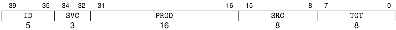
Figure 5.2: BrLite message header (40 bits). The total flit length is 80 bits with the 40-bit payload.
