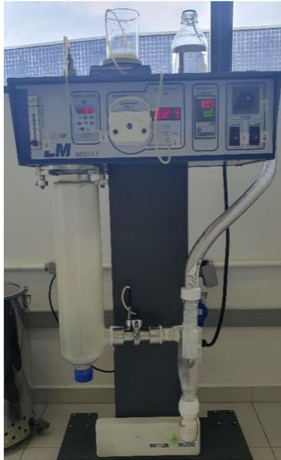
Figura 4.3. *Spray dryer* LabMat MSD 0.5.
