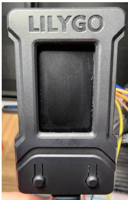
Figura 4 - ESP32 TTGO LCD 1.14"
