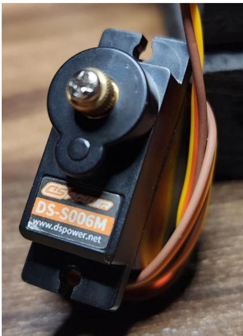
Figura 9 – Servomotor Digital 12g
