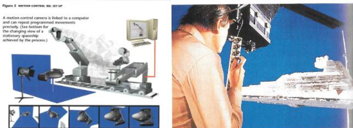
Figura 28 – Motion control set-up e Dennis Muren filmando The Empire Strikes Back (1980)
