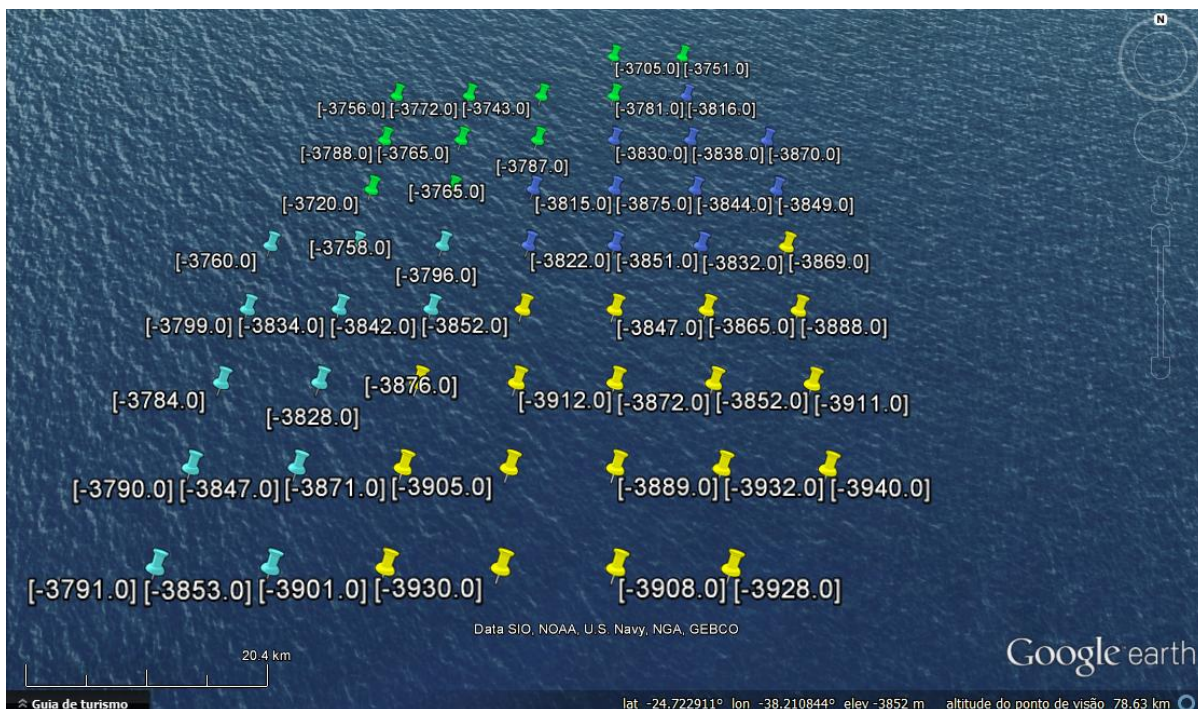
Figure 30 - KML file plotted on Google Earth showing clusters formed using Euclidean formula on the selected area of filtered noaa_bathymetry dataset. Cluster 1 is identified by yellow color; cluster 2 is identified by blue color. Values are bathymetry of each respective point.
